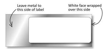
Smallest recommended bending diameter of the Confidex Steelwave Flex<sup>™</sup> is 50mm. For optimal read range please bend the label in the orientation shown below. Note that with smaller assets it is recommended to bend the label to other direction for optimal adhesion.
