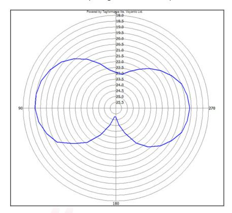
Angular Sensitivity (Relative Read Range vs. Orientation)
