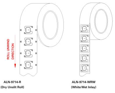
Standard Alien Inlay rolls unwind with metal antenna side facing outward, with respect to the core.
