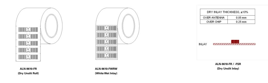
Standard Alien Inlay rolls unwind with metal antenna side facing outward, with respect to the core.
