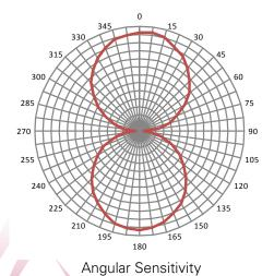
Angular Sensitivity (Relative Read Range vs. Orientation)
